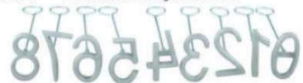
01-1024 Aluminum Paint Branding Irons 9.00 $ Made of aluminum castings, light in weight. Set consists of nine irons in 2.5" sizes. 0.5" depth, 1.5" width. Also available in 4" sizes. NOTE: A set 0-9 does not include the figure 9. The 6 iron can be reversed to make the figure 9.
