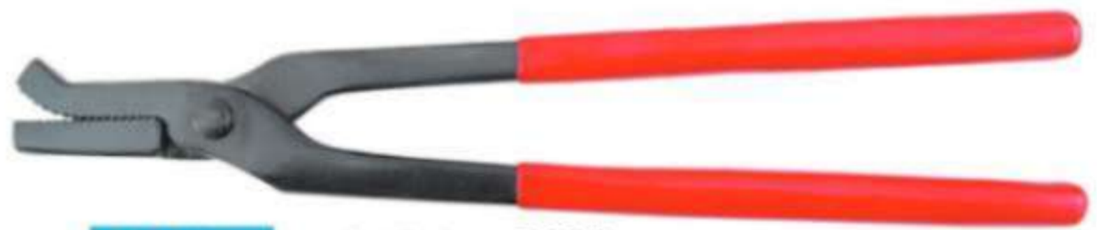
01-1105 Farrier Clincher 7.50 $ To roll over nails with curved jaw. Red vinyl coated handle gives a comfortable grip. Length 13" c/s. Also available in stainless steel.
